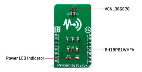
The VCNL36687S features a 12-bit ADC, therefore the output data is in 12-bit format. There are two registers that are used to hold the output result. Besides the four Most Significant Bits (MSBs), the PS data output high-byte register contains another bit that indicates that the device entered the sunlight protection mode.
