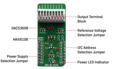
The DAC 5 click has a high precision voltage reference included onboard. For that purpose, MAX6106 is used, a 2.048V voltage reference IC, from Maxim Integrated. This little SOT23 device is stable with capacitive loads, and no output capacitor is required. It has regulations for both sink and source and is very accurate. This gives DAC 5 click good flexibility for use in various applications.
