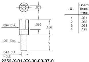
**Description:** 2352 - Slotted Terminal Pin Packaging: Packaged in Bulk
