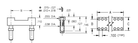
DIP Dual In Line Receptacle Carrier Socket Plastic DIP Carrier with Low Profile Receptacles Open Frame **Plating Code:** 91 **Shell Plating:** 200  $\mu$ " Tin/Lead(93/7) over 100  $\mu$ " Nickel **Inner Contact Plating:** 10  $\mu$ " Gold over 50  $\mu$ " Nickel **Packaging:**
