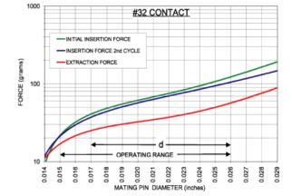
The insertion/extraction/normal force characteristics above were derived using a 30 microinch gold plated contact and polished steel gauge pins having a bullet-shaped tip.
