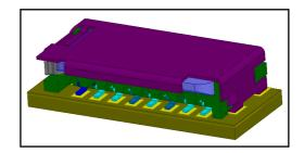
SD card constructed on polycarbonate has a finished board thickness of 0.7mm. It includes micro-strip of 0.1mm x 0.9mm with stack height of 0.374mm, and gold fingers of 3.6mm x 0.9mm without ground reference under these pads.
