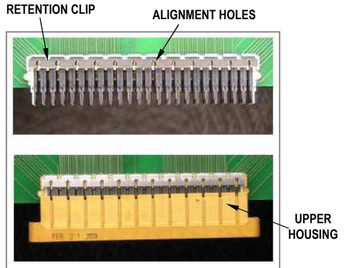
8. Install the retention clip to the lower housing by aligning the holes in the stiffener to the bosses in the lower housing. While holding the stiffener in place, slide the upper housing on until it just starts to engage the stiffener. See Figure 7.
