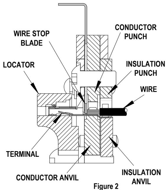
3. Place a pre-stripped wire into the terminal and align the wire with the conductor and insulation grips visually. See Figure 2 and 3.
