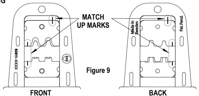
2. Remove the M3 BHCS which is holding the upper tooling. Flip the upper tooling to the opposite side and replace the M3 BHCS. Make sure the small markings on the front and back of the hand tool frame, match up and are on the outside of the hand tool frame. See Figure 8 and 9.
