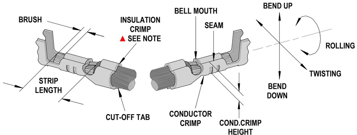
This illustration is a generic terminal representation and not an exact image of any terminal listed in the scope.
