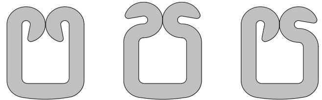
This crimp terminal is designed for miniaturization; therefore, each dimension of insulation crimp portion appears small as compared to the terminal material thickness. In order to avoid insulation piercing the crimp forms by the insulation barrel, coining is provided inside of the insulation barrel. For this reason, various crimp forms will occur at the tip of the insulation crimp barrel shown in the figure below.
