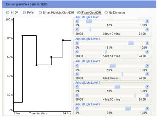
Allow users to separate 24hrs into 5 sections and corresponding output current.
