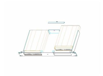
3. Mount the BA2X1U in your 19' rack using the mounting screws that match your rack's thread size. Follow the rack manufacturer's documentation to safely and securely mount the BA2X1U in the 19' rack.
