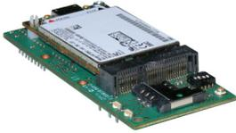
The SocketModem<sup>®</sup> Cell cellular modem is a complete, ready-to-integrate communications device that offers standards-based quad-band HSPA 7.2 performance. This quick-to-market communications device allows developers to add wireless communication to products with a minimum of development time and expense. The SocketModem Cell cellular modem is based on industry-standard open interfaces and utilizes Multi-Tech's Universal Socket design.
