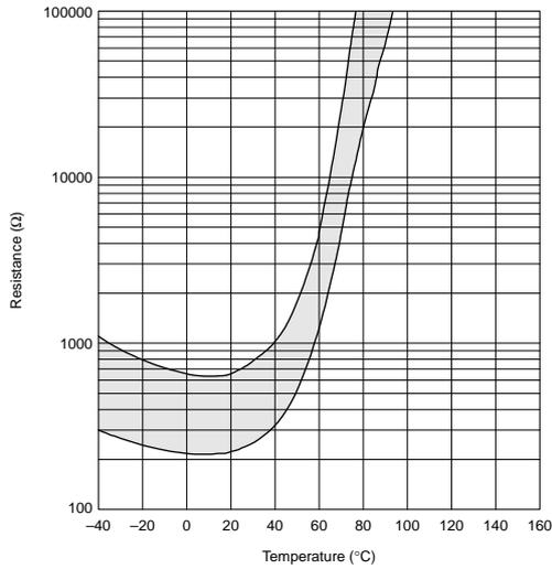
■ Resistance - Temperature Characteristics Range (Ref. Only) Tight Tolerance Type
