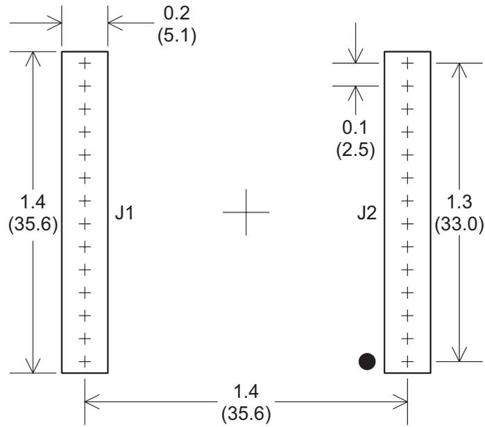
Connectors are FCI Electronics 66951-014 or equivalent
