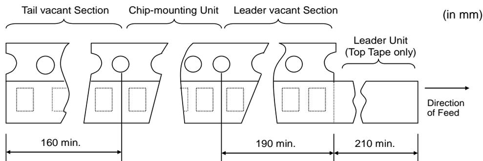
1.5 Accumulate pitch : 10 of sprocket holes pitch =  $40 \pm 0.3\text{mm}$
