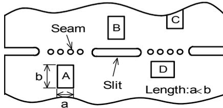
\*1  $A > D$  is valid when stress is added vertically to the perforation as with Hand Separation.
