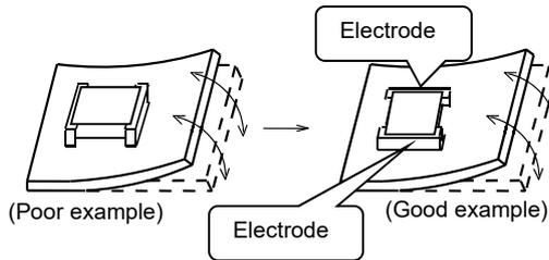
(2) Components location on PCB separation
