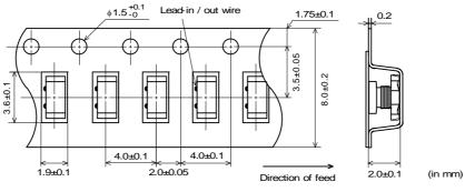
$\mbox{\cdot}\mbox{Dimension}$  of the Cavity is measured at the bottom side.
