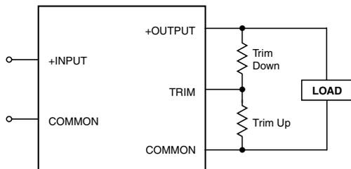
Note: Install either a fixed trim-up resistor or a fixed trim-down resistor depending upon desired output voltage.
