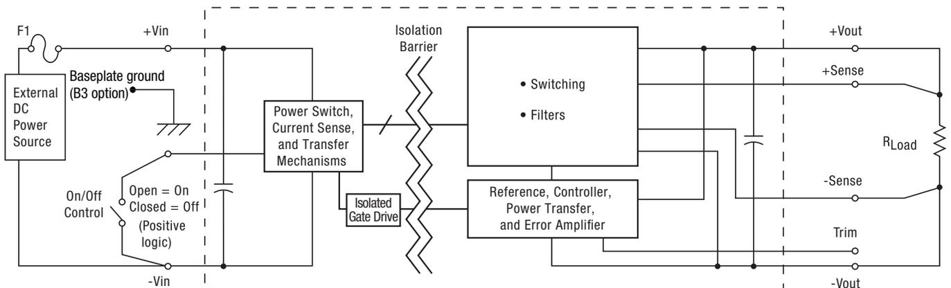
Figure 1. Connection Diagram
