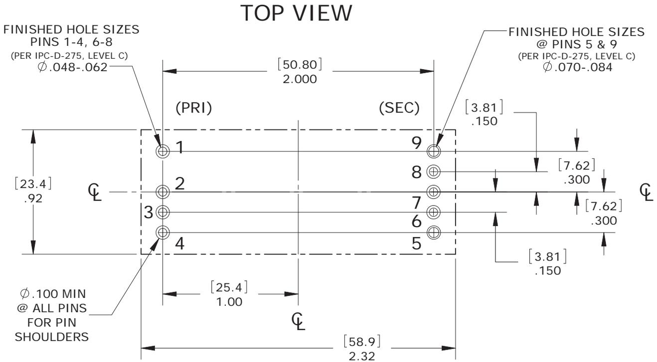
IT IS RECOMMENDED THAT NO PARTS BE PLACED BENEATH CONVERTER (HATCHED AREA)
