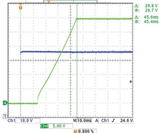
Enable Start up Delay (Vin = 48V, Vout = nom, Iout = full load, Ta = +25°C)
