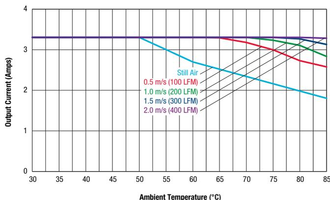
Maximum Current Temperature Derating at sea level (V<sub>in</sub> = 36V, airflow from pin 1 to pin 4, with baseplate)
