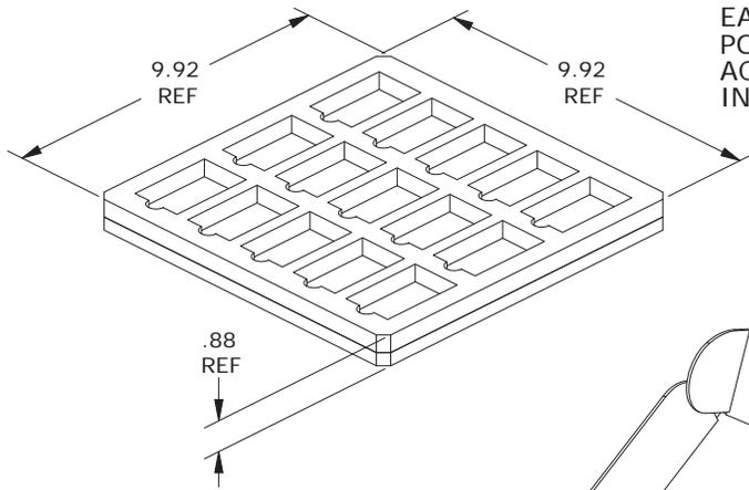
EACH STATIC DISSIPATIVE POLYETHYLENE FOAM TRAY ACCOMMODATES 15 CONVERTERS IN A 3 X 5 ARRAY
