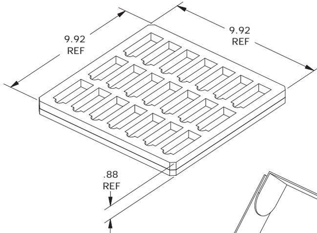
EACH STATIC DISSIPATIVE POLYETHYLENE FOAM TRAY ACCOMMODATES 21 CONVERTERS IN A 3 X 7 ARRAY
