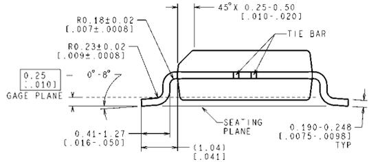
CONTROLLING DIMENSION IS MILLIMETER
