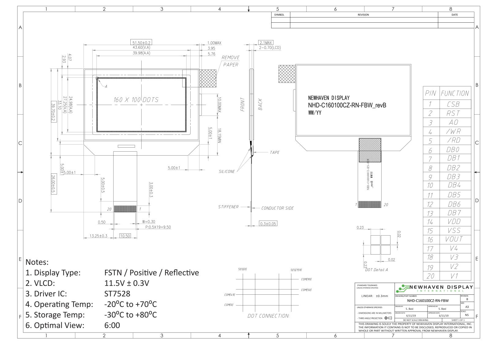
**Pin Description and Wiring Diagram**
