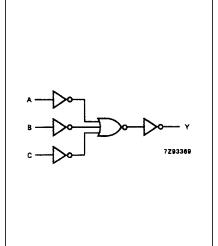
Fig.5 Logic diagram (one gate).
