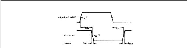
(1) HC :  $V_M$  = 50%;  $V_I$  = GND to  $V_{CC}$ . HCT:  $V_M$  = 1.3 V;  $V_I$  = GND to 3 V.
