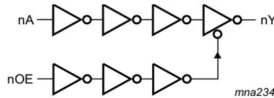
Fig 3. Logic diagram (one buffer/line driver)
