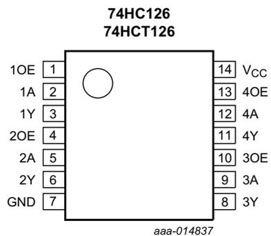
Fig 5. Pin configuration for SOT337-1 and SOT402-1
