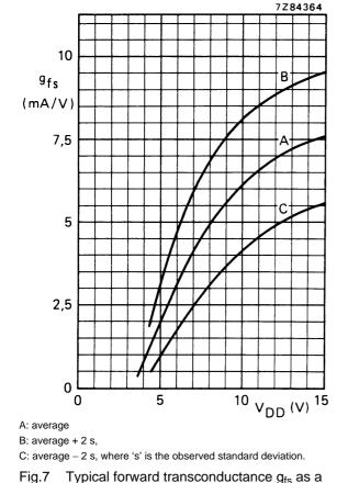
Typical forward transconductance gfs as a function of the supply voltage at T<sub>amb</sub> = 25 °C.
