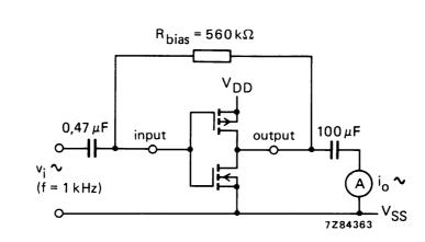
Fig.6 Test set-up for measuring forward transconductance  $g_{fs} = di_o/dv_i$  at  $v_o$  is constant (see also graph Fig.7); MR = LOW.
