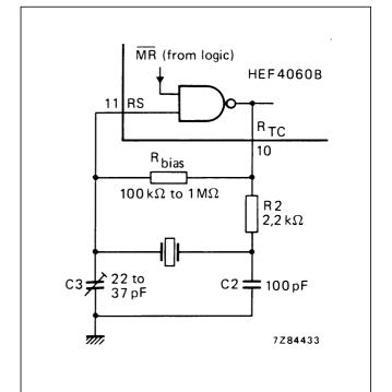
Fig.5 External component connection for crystal oscillator.
