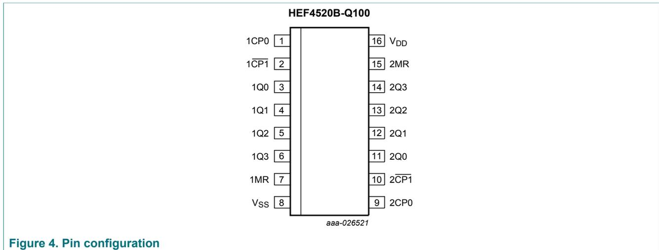
Figure 4. Pin configuration
