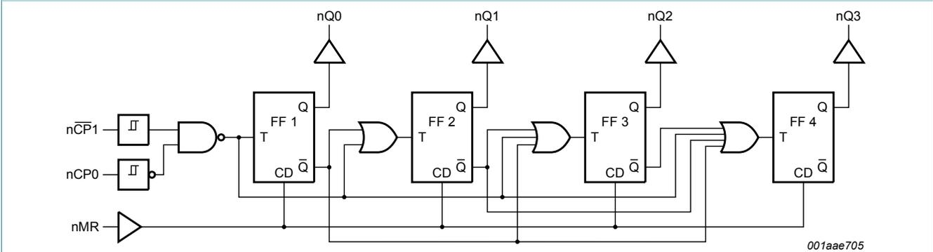
Figure 3. Logic diagram for one counter
