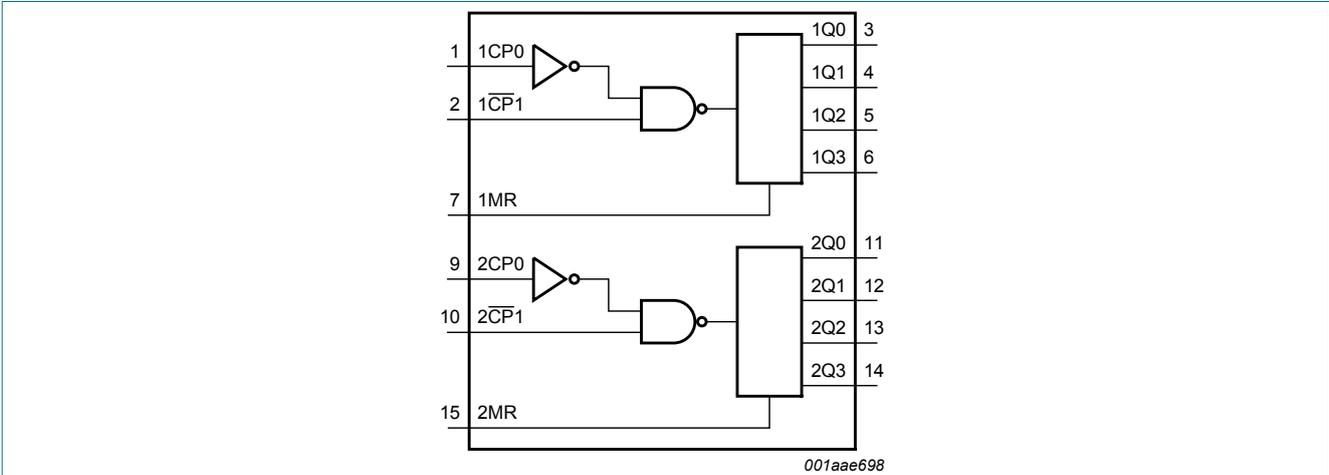
Figure 1. Functional diagram
