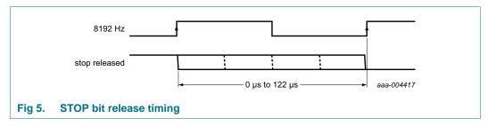
The first increment of the time circuits is between 0.507813 s and 0.507935 s after STOP bit is released. The uncertainty is caused by the prescaler bits  $F_0$  and  $F_1$  not being reset (see <u>Table 7</u>) and the unknown state of the 32 kHz clock.
