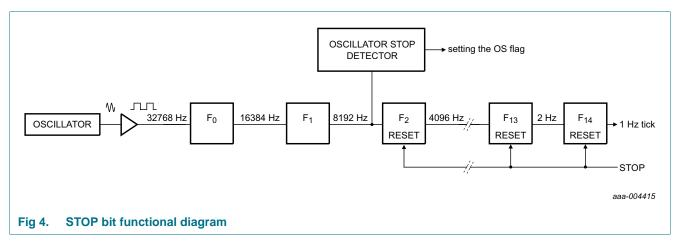
The time circuits can then be set and do not increment until the STOP bit is released (see Figure 5 and Table 7).
