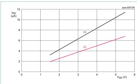
$T_{amb}$  = 25 °C;  $f_{CLKOUT}$  = 32768 Hz.
