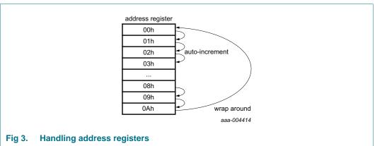
All 11 registers (see Table 5) are designed as addressable 8-bit parallel registers although not all bits are implemented. The first two registers (memory address 00h and 01h) are used as control and status register. The register at address 02h is an offset register allowing the fine-tuning of the clock; and at 03h is a free RAM byte. The addresses 04h through 0Ah are used as counters for the clock function (seconds up to years counters).
