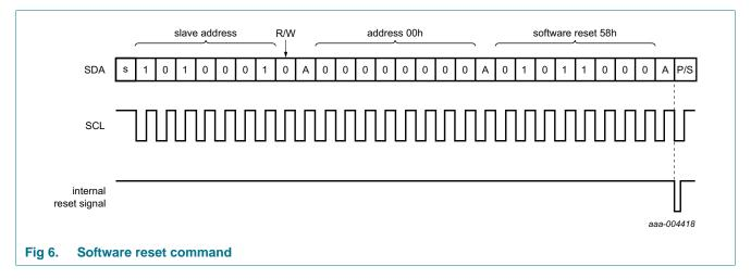
In reset state all registers are set according to <u>Table 8</u> and the address pointer returns to address 00h.
