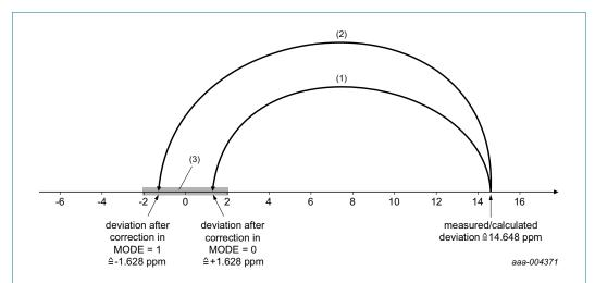
With the offset calibration an accuracy of  $\pm 2$  ppm (0.5 × offset per LSB) can be reached (see Table 13).
