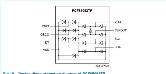
Fig 19. Device diode protection diagram of PCF85063TP
