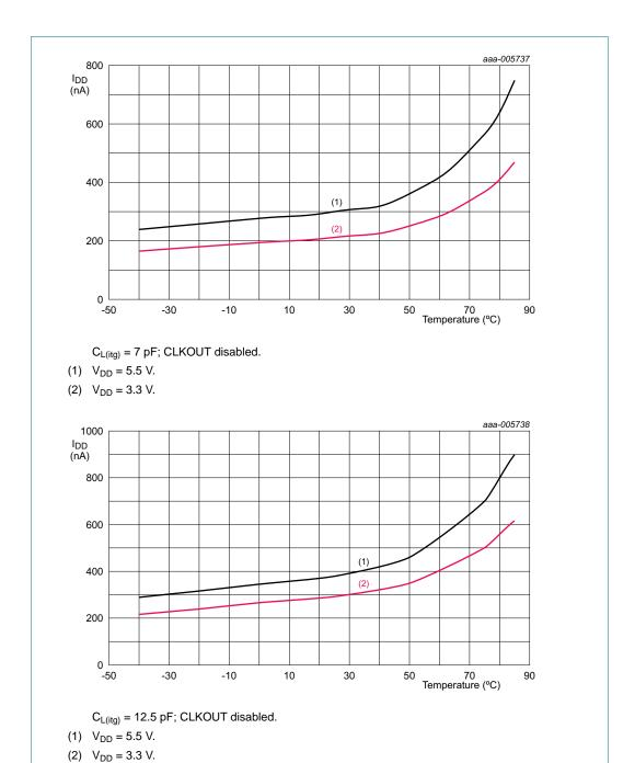
Fig 21. Typical  $I_{DD}$  as a function of temperature
