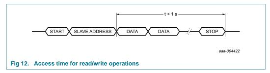
Because of this method, it is very important to make a read or write access in one go, that is, setting or reading seconds through to years should be made in one single access. Failing to comply with this method could result in the time becoming corrupted.
