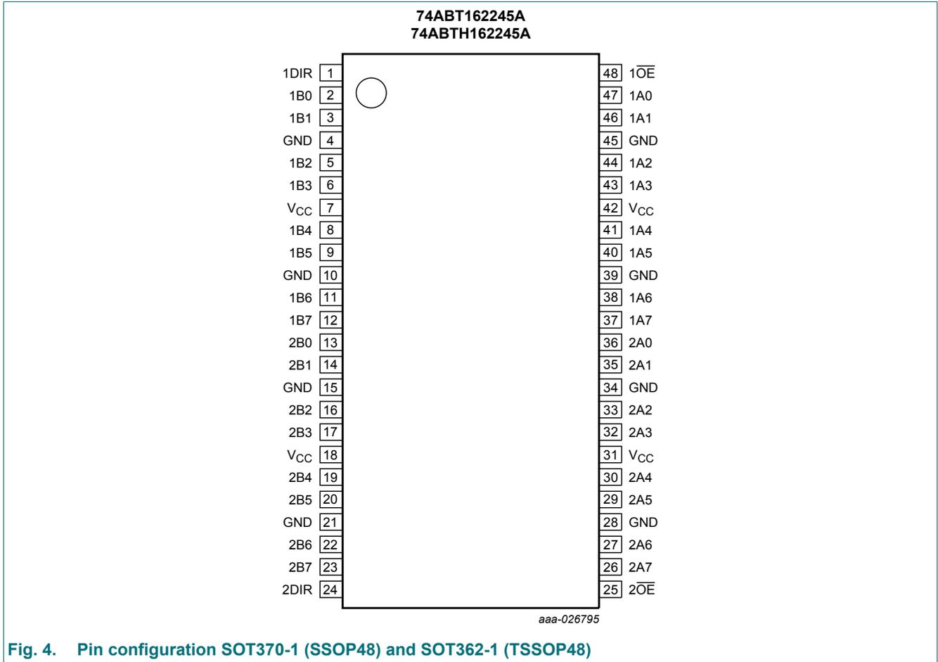
Fig. 4. Pin configuration SOT370-1 (SSOP48) and SOT362-1 (TSSOP48)
