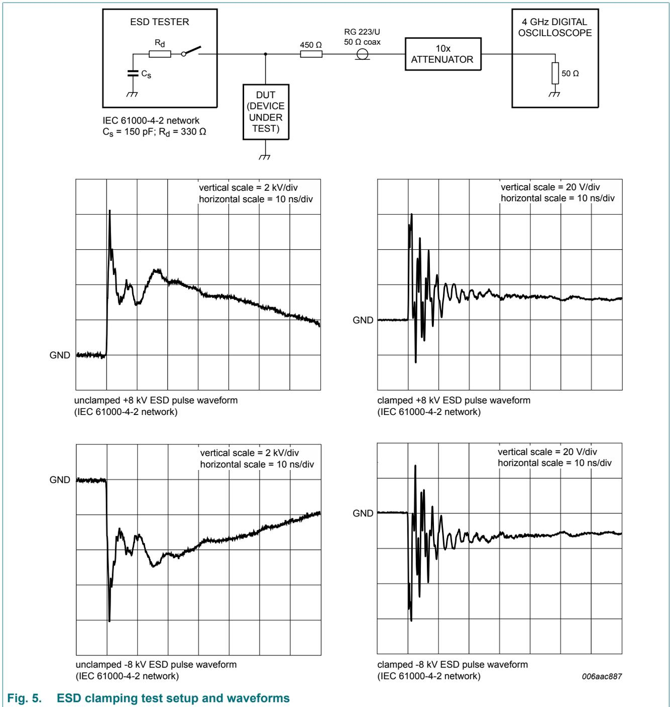
Fig. 5. ESD clamping test setup and waveforms
