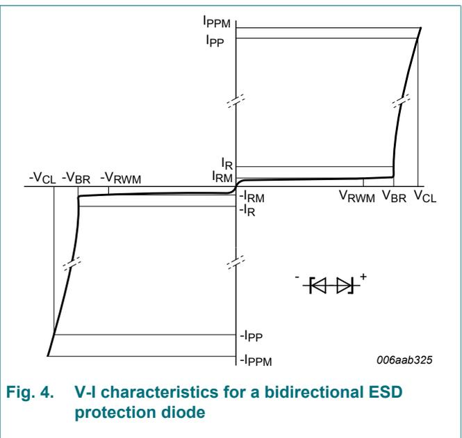
Extremely low capacitance bidirectional ESD protection diode
