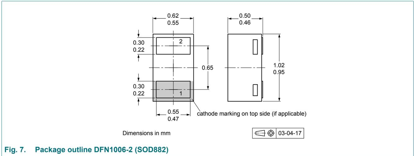
Fig. 7. Package outline DFN1006-2 (SOD882)
