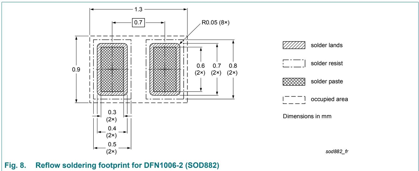
Fig. 8. Reflow soldering footprint for DFN1006-2 (SOD882)
