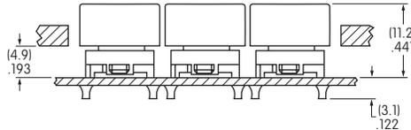
Custom keyboards can be designed with caps installed through a panel cutout (illustration with cap AT4060).
