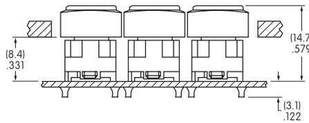
Custom keyboards can be designed with caps installed through a panel cutout (illustration with cap AT4076).
