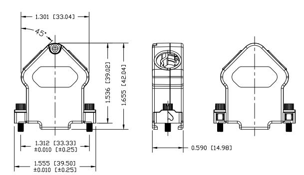
MATERIAL: DIE-CAST ZINC ALLOY PLATING: NICKEL OVER COPPER JACKSCREWS: STEEL, ZINC PLATED STEEL, ZINC PLATED COVER PLATE: STEAL, ZINC PLATED STEAL, ZINC PLATED STEAL, ZINC PLATED STEAL, ZINC PLATED STEEL, ZINC PLATED
