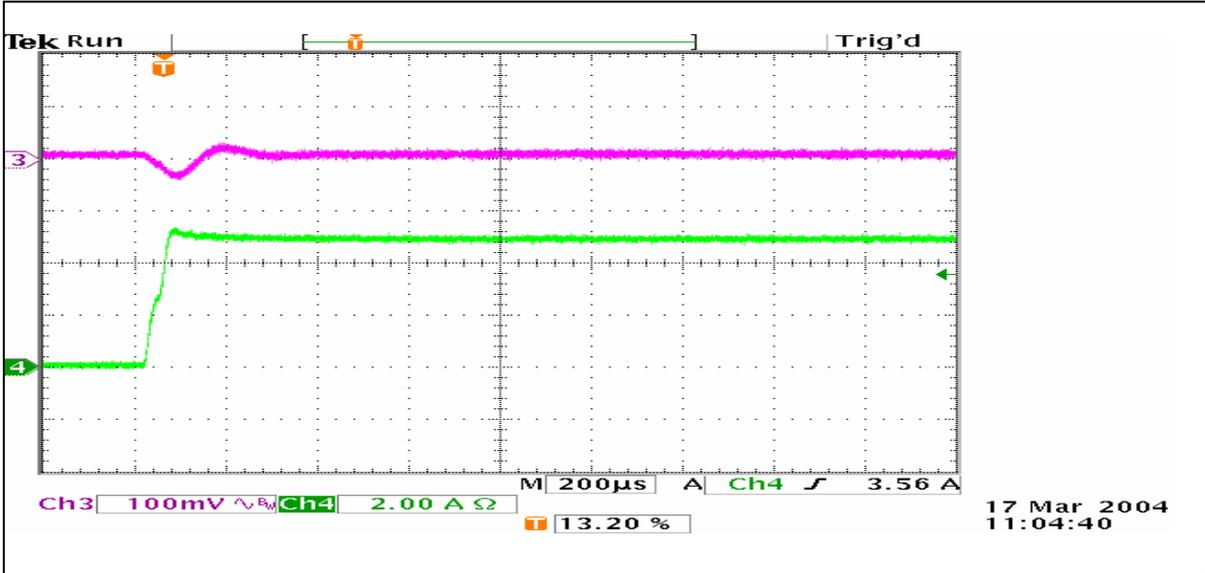
Load Transient: VCC=5V; VOUT=2.5V; Cout=2200uF
