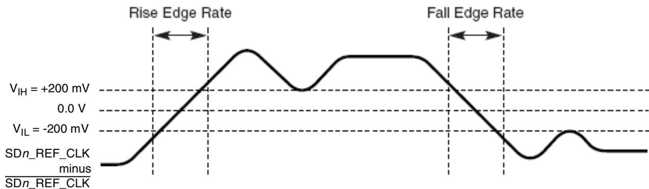
**Figure 52. Differential Measurement Points for Rise and Fall Time**
