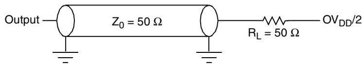
Figure 40. I<sup>2</sup>C AC Test Load
