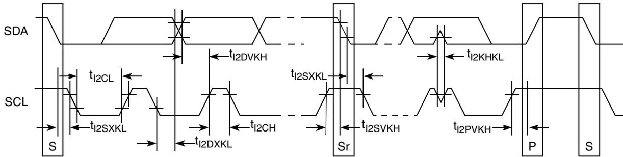
Figure 41. I<sup>2</sup>C Bus AC Timing Diagram
