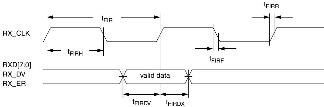
Figure 8. FIFO Receive AC Timing Diagram
