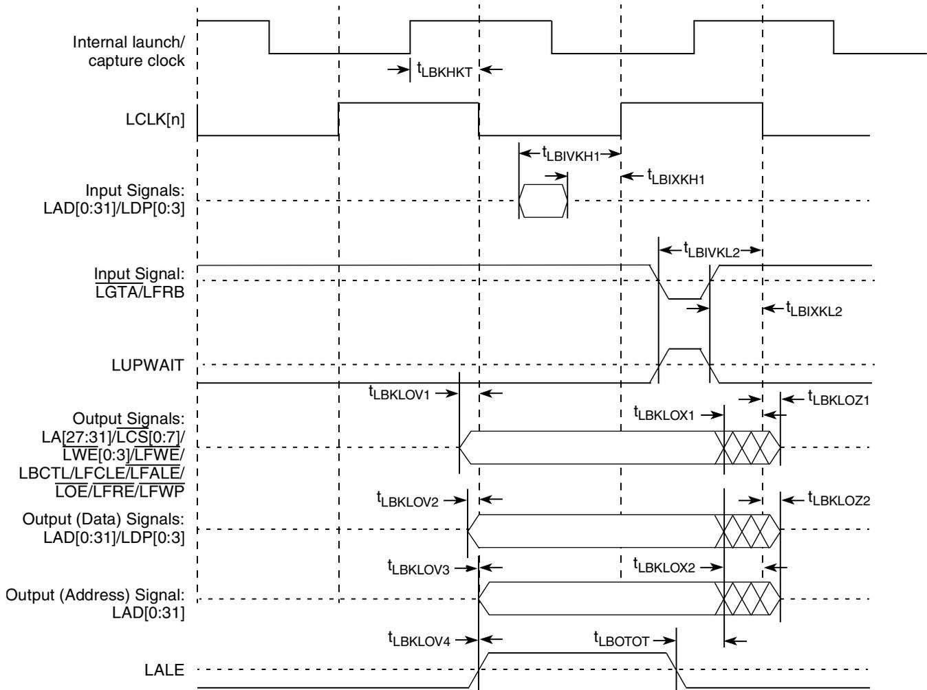
**Figure 31. Local Bus Signals (PLL Bypass Mode)**
