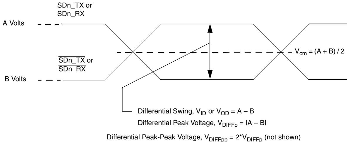
**Figure 43. Differential Voltage Definitions for Transmitter or Receiver**
