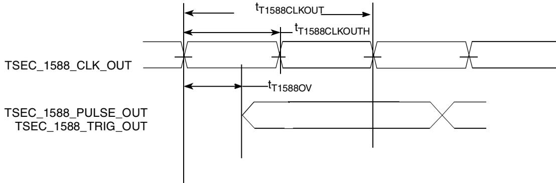
Figure 26. eTSEC IEEE 1588 Output AC Timing
