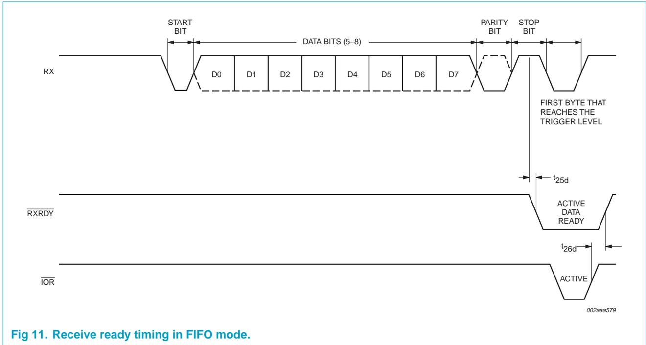
Fig 11. Receive ready timing in FIFO mode.
