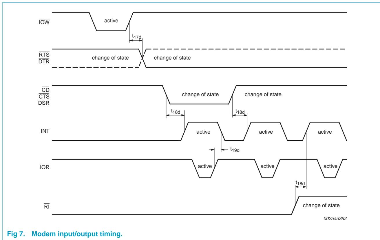
Fig 7. Modem input/output timing.
