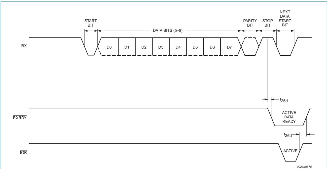
Fig 10. Receive ready timing in non-FIFO mode.
