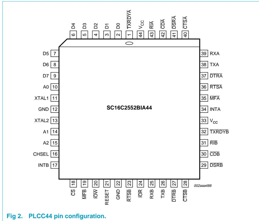
Fig 2. PLCC44 pin configuration.
