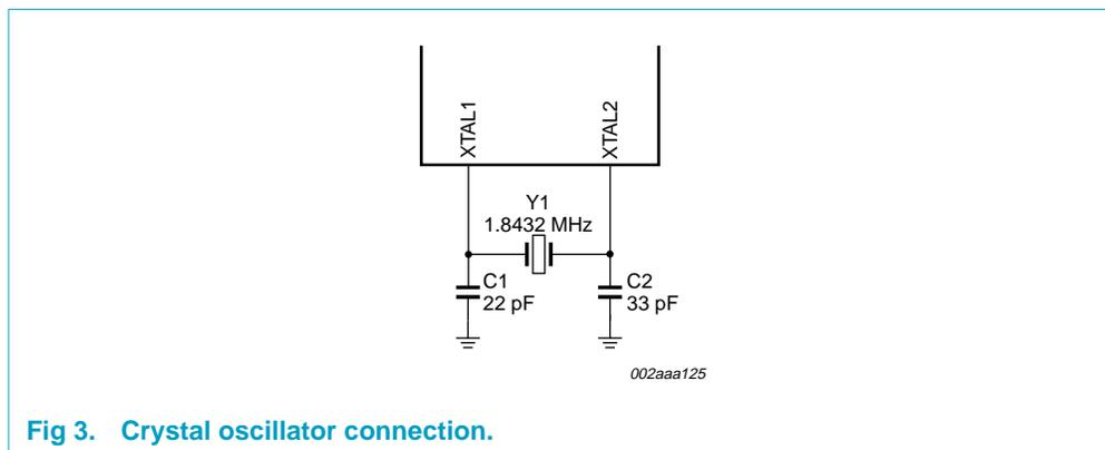
Fig 3. Crystal oscillator connection.
