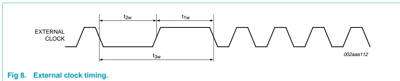
Fig 8. External clock timing.
