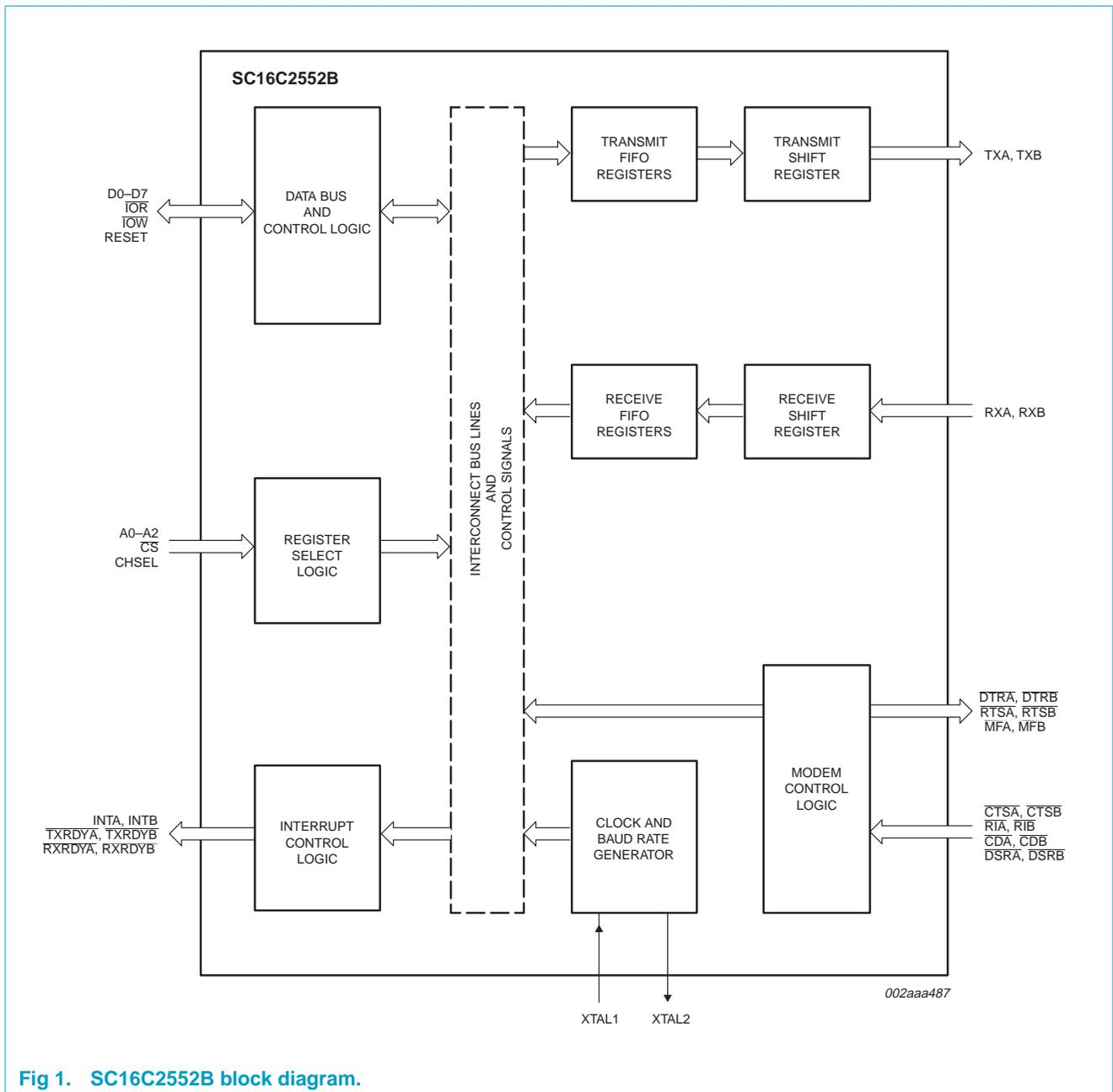
Fig 1. SC16C2552B block diagram.
