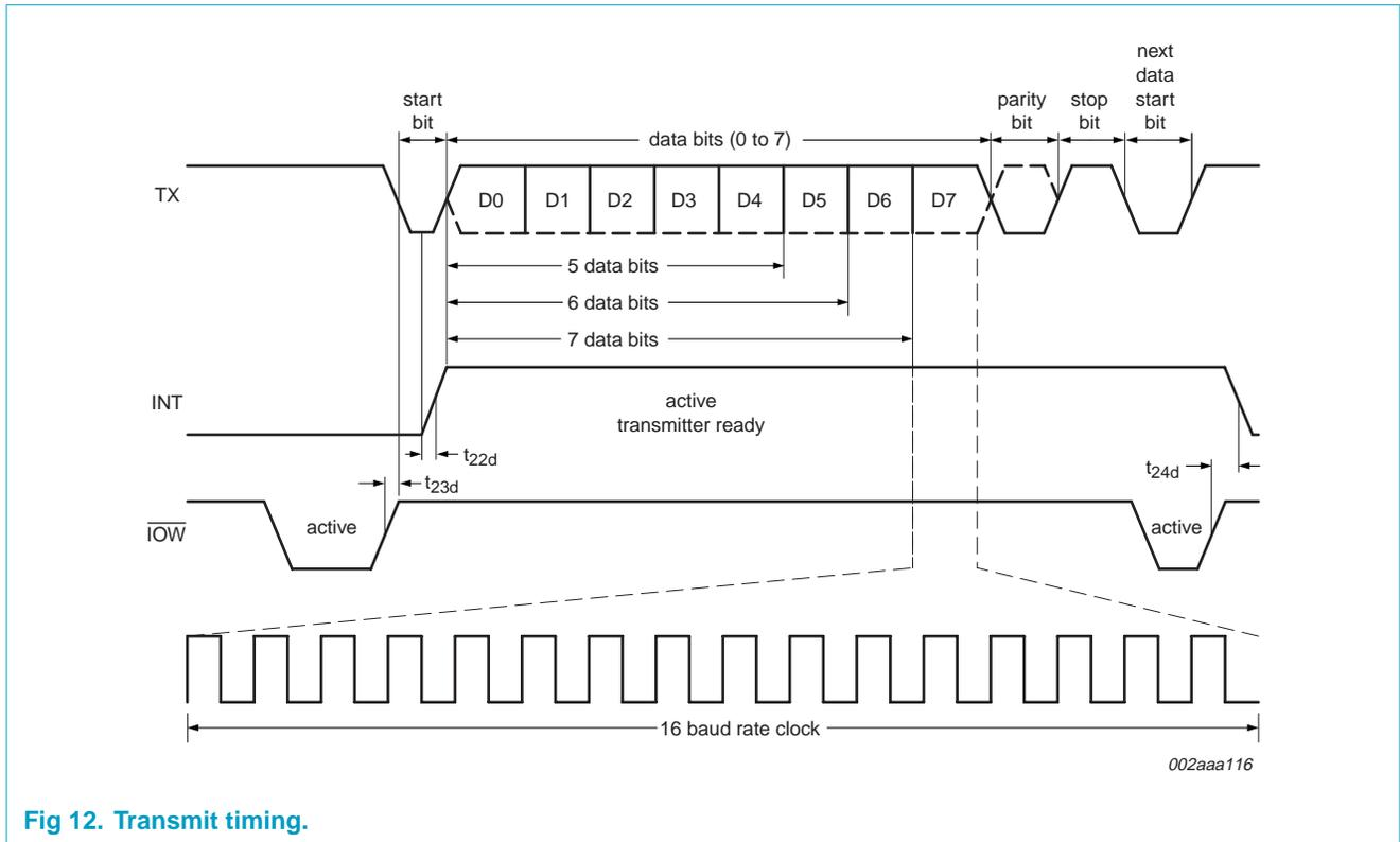
Fig 12. Transmit timing.
