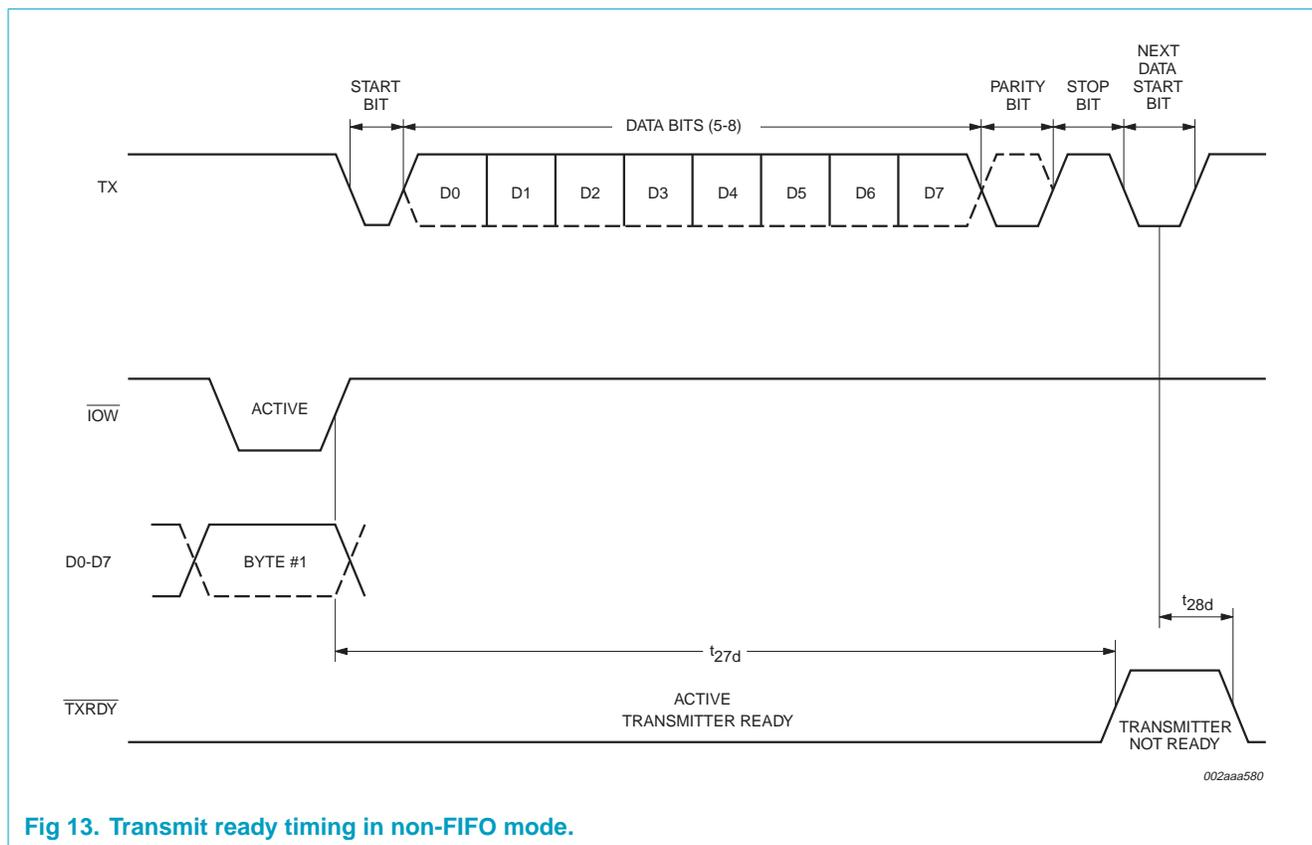
Fig 13. Transmit ready timing in non-FIFO mode.
