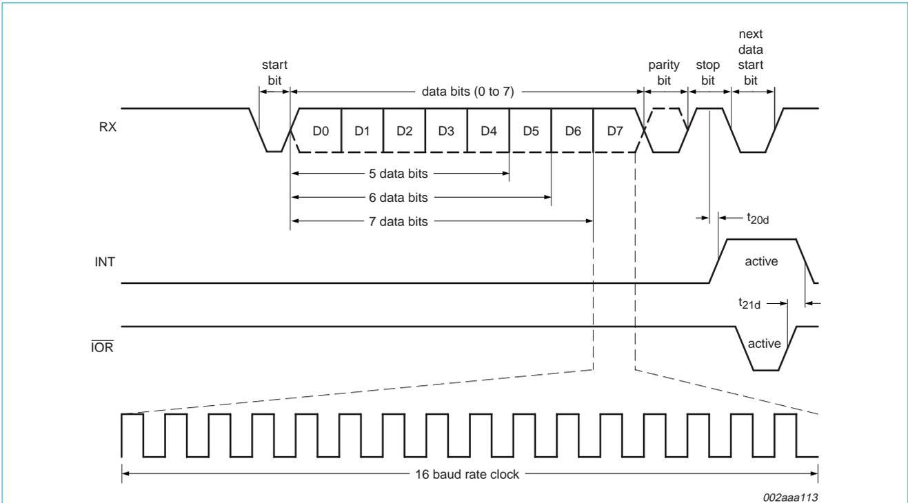
Fig 9. Receive timing.
