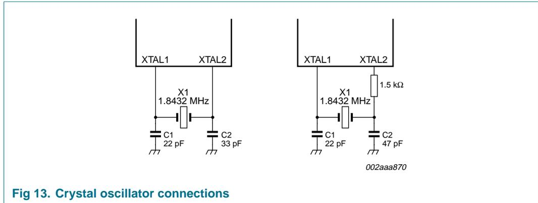
Fig 13. Crystal oscillator connections
