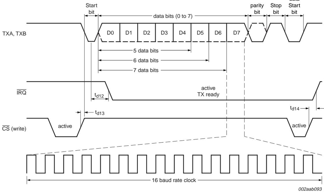
Fig 21. Transmit timing
