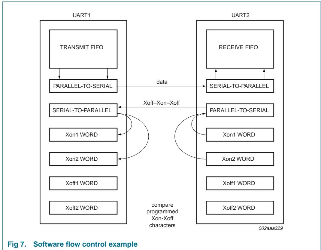
Fig 7. Software flow control example
