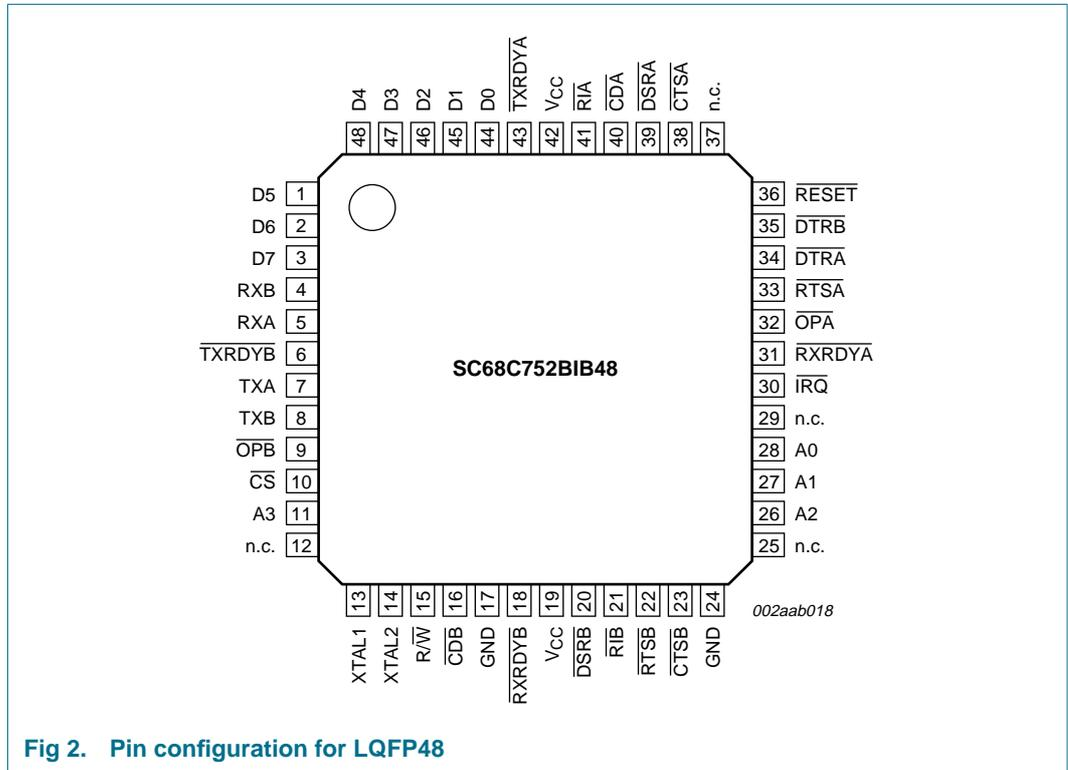
Fig 2. Pin configuration for LQFP48
