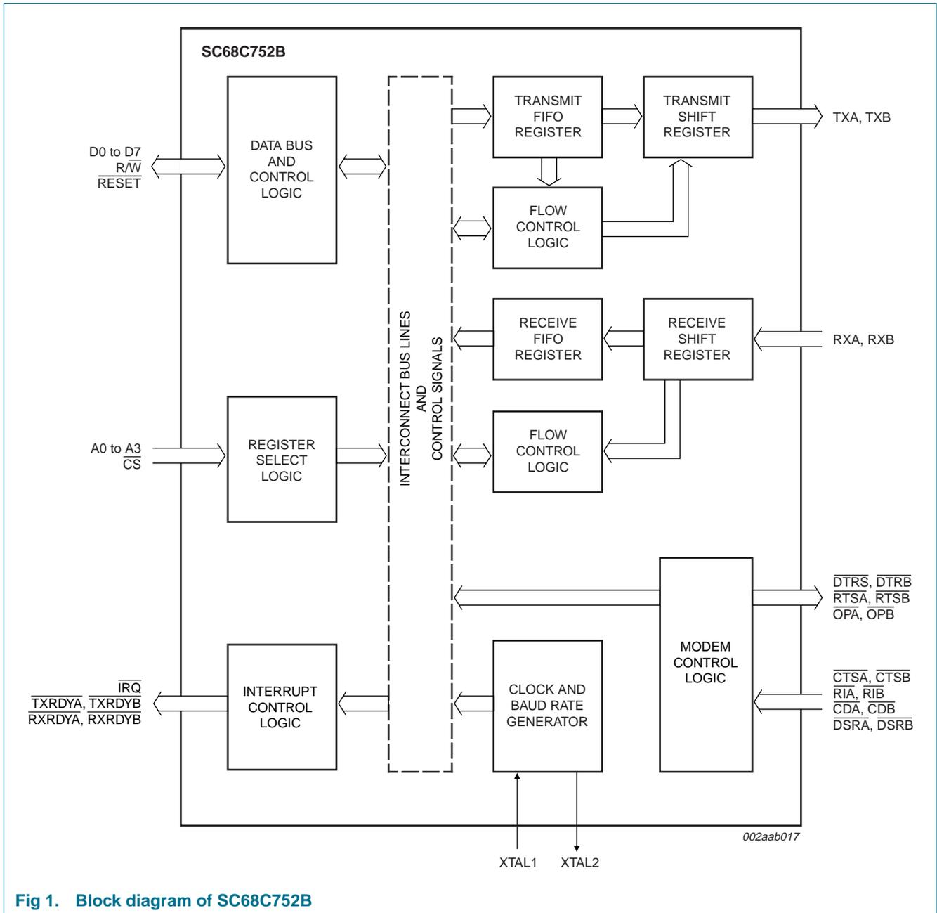
Fig 1. Block diagram of SC68C752B
