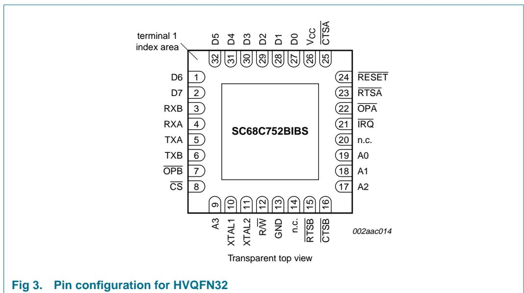
Fig 3. Pin configuration for HVQFN32
