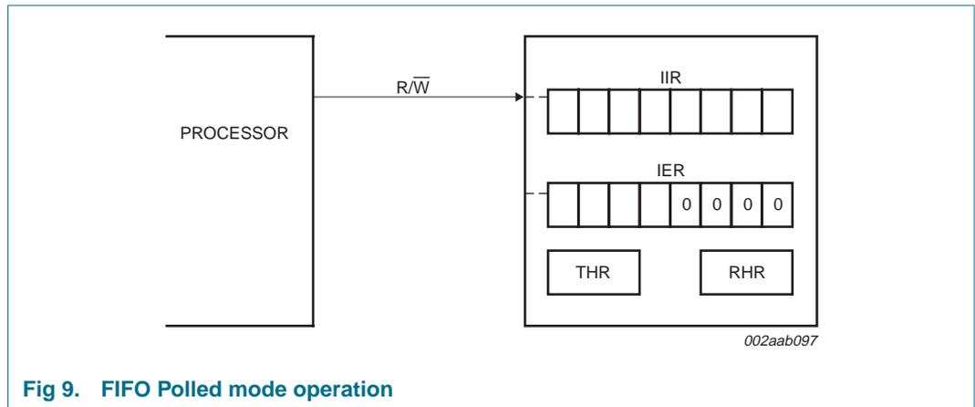
Fig 9. FIFO Polled mode operation
