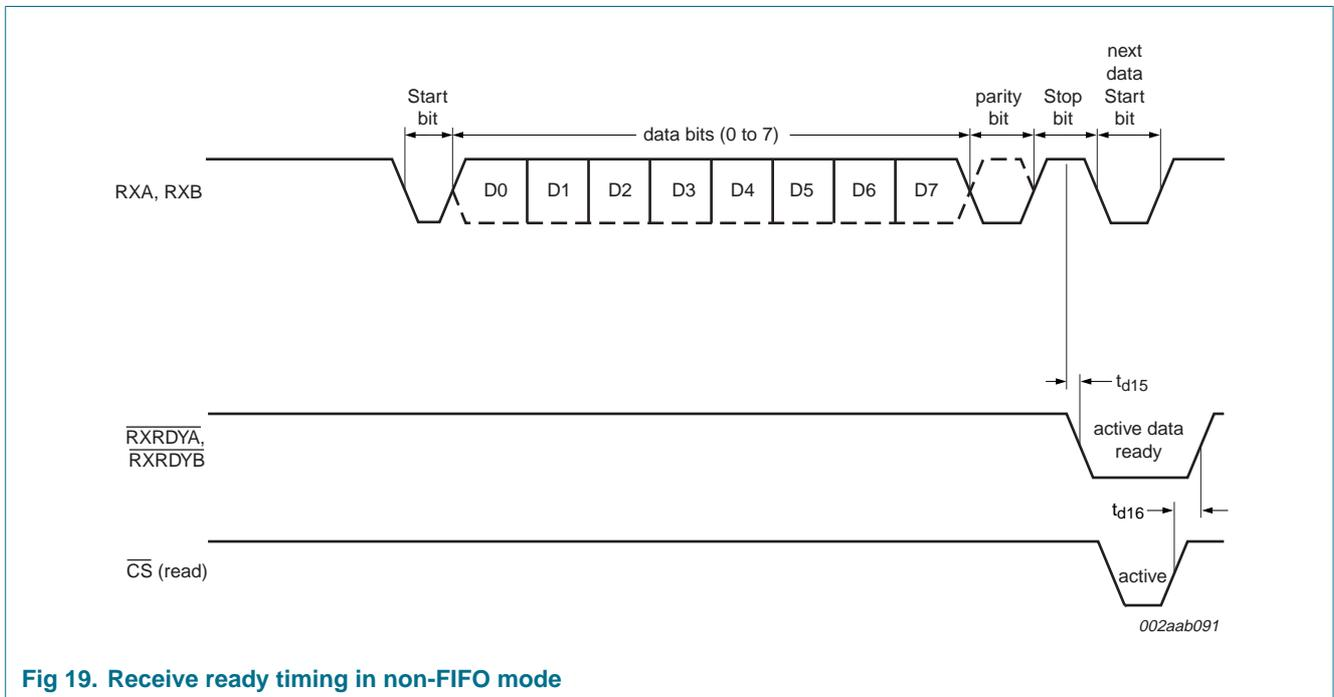
Fig 19. Receive ready timing in non-FIFO mode
