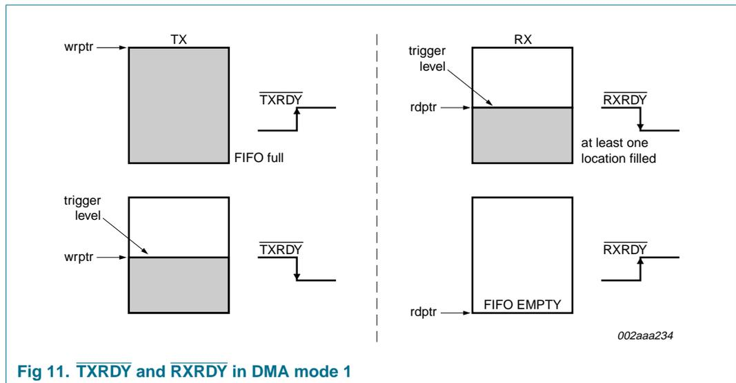
Fig 11.  $\overline{\text{TXRDY}}$  and  $\overline{\text{RXRDY}}$  in DMA mode 1
