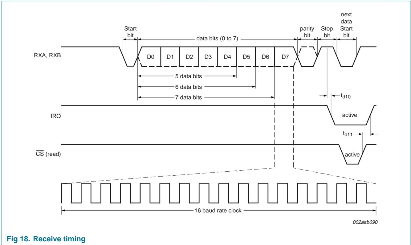
Fig 18. Receive timing
