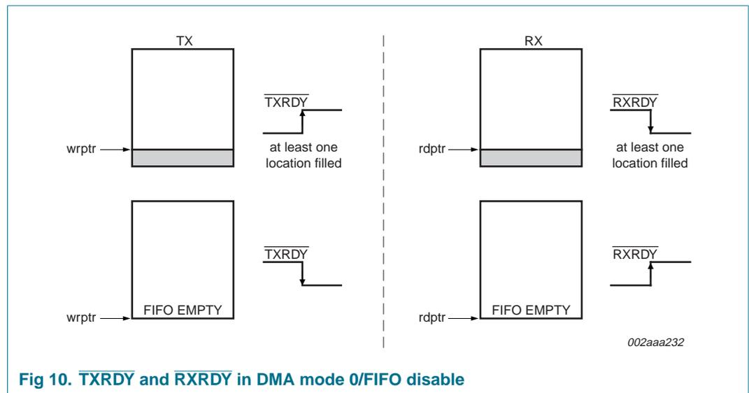
Fig 10.  $\overline{\text{TXRDY}}$  and  $\overline{\text{RXRDY}}$  in DMA mode 0/FIFO disable
