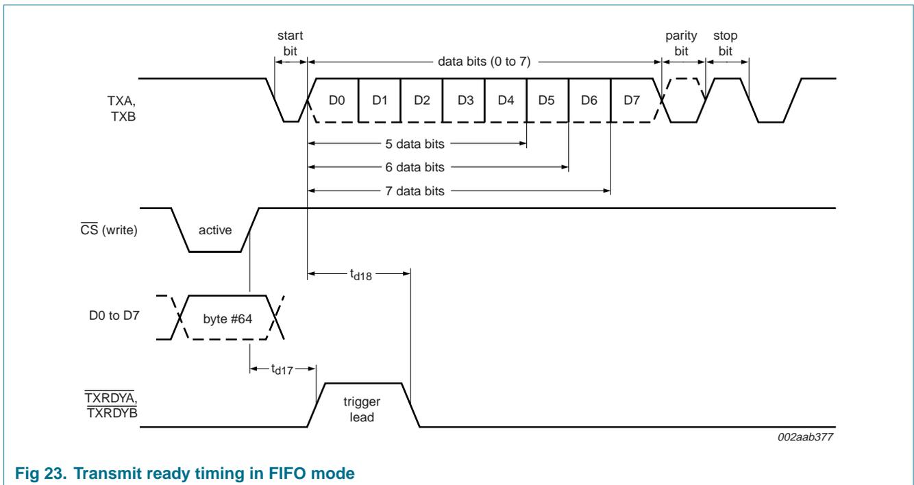
Fig 23. Transmit ready timing in FIFO mode
