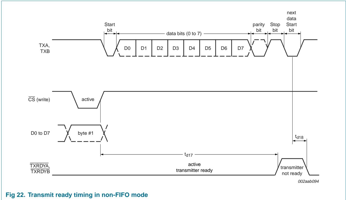
Fig 22. Transmit ready timing in non-FIFO mode
