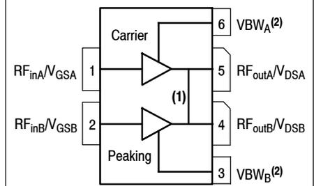
**Figure 1. Pin Connections**
