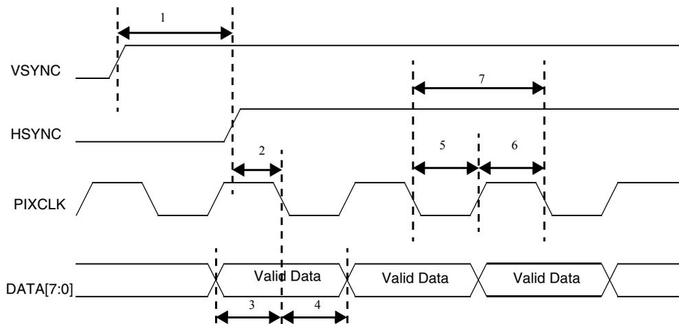
**Figure 82. Sensor Output Data on Pixel Clock Rising Edge
