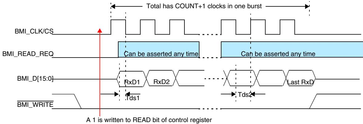
**Figure 9. BMI Drives Clock, MMD Write BMI Timing**
