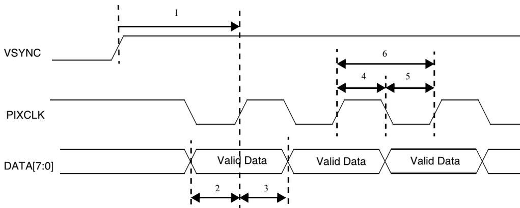
**Figure 83. Sensor Output Data on Pixel Clock Falling Edge
