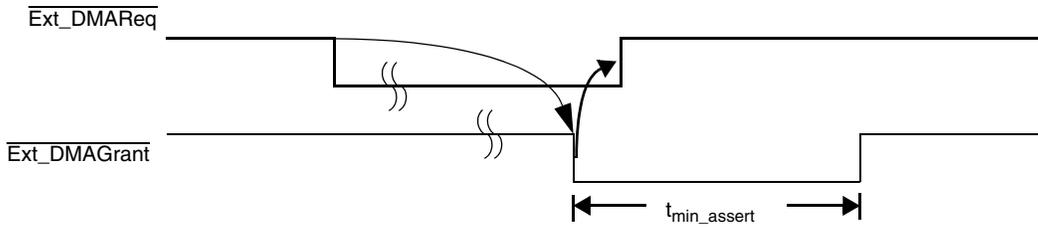
**Figure 4. Assertion of DMA External Grant Signal**
