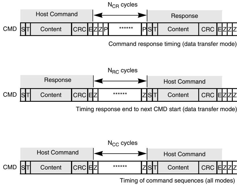
**Figure 27. Timing Diagrams at Data Transfer Mode**
