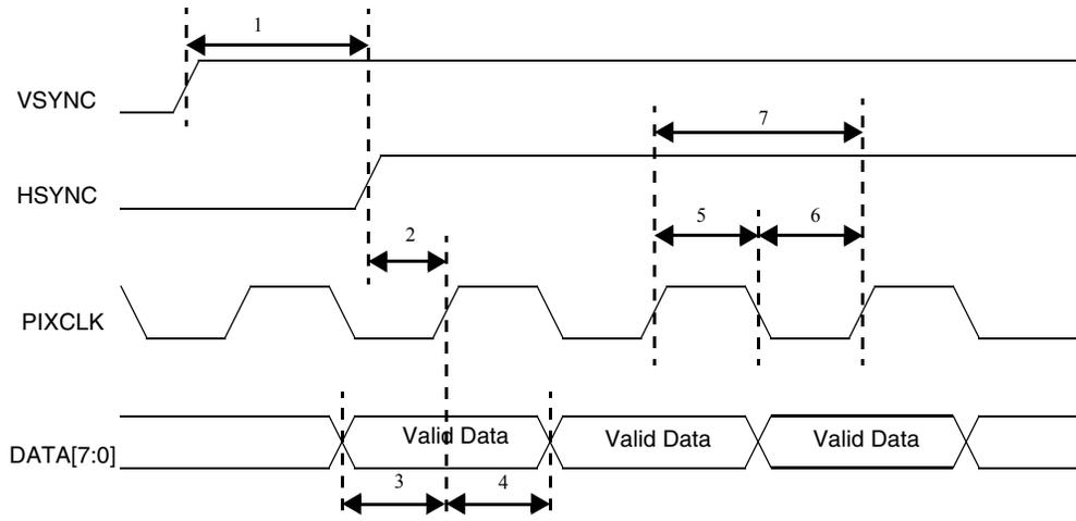
**Figure 81. Sensor Output Data on Pixel Clock Falling Edge
