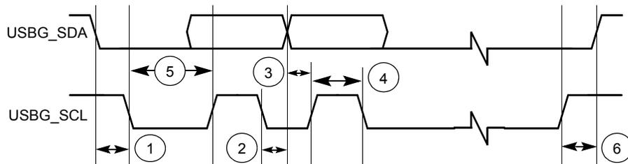
Figure 52. USB Timing Diagram for Data Transfer from USB Transceiver (I<sup>2</sup>C)
