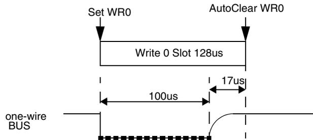
**Figure 47. Write 0 Timing**
