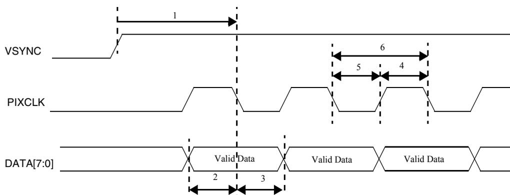
**Figure 84. Sensor Output Data on Pixel Clock Rising Edge
