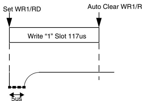
**Figure 48. Write 1 Timing**
