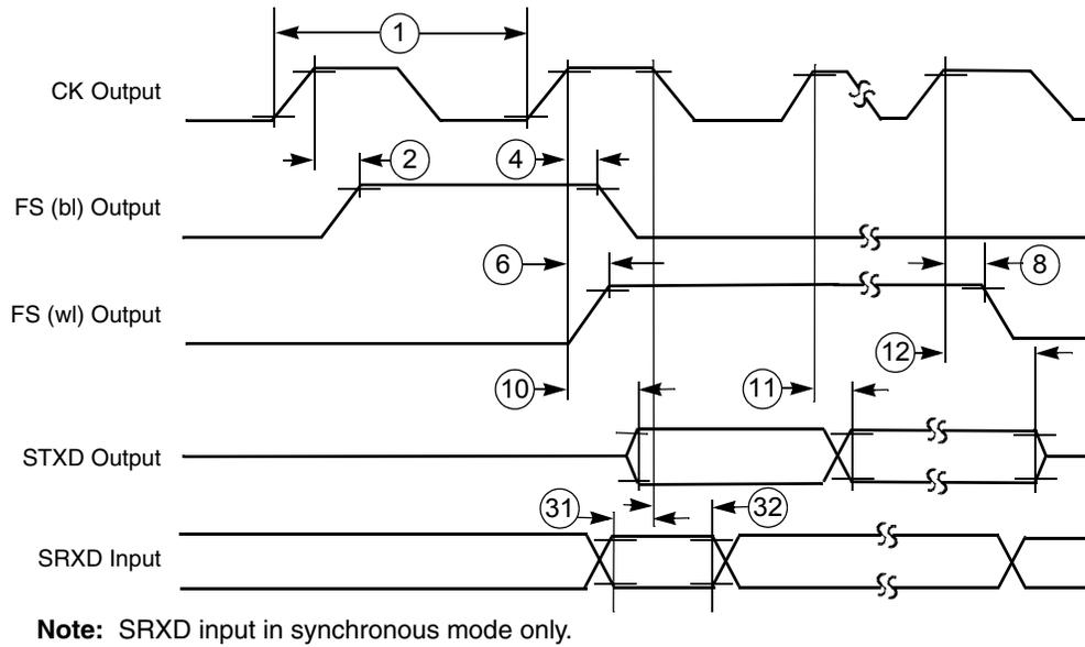
**Figure 42. SSI Transmitter Internal Clock Timing Diagram**
