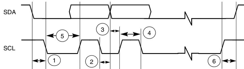
Figure 80. Definition of Bus Timing for I<sup>2</sup>C
