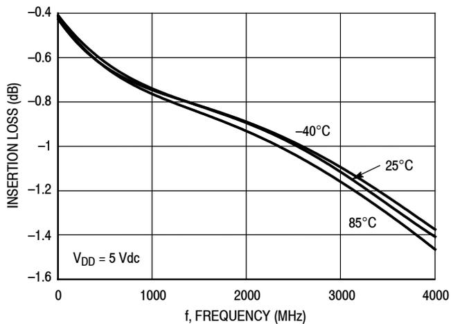
Figure 5. Insertion Loss versus Frequency versus Temperature
