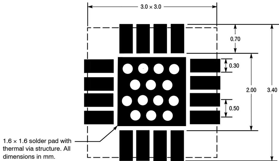
Figure 13. PCB Pad Layout for QFN 3 x 3, 16 Lead
