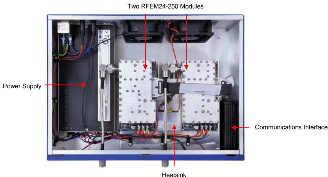
**Figure 3. RFEL24-500 RF Energy Lab Box – Internal View**
