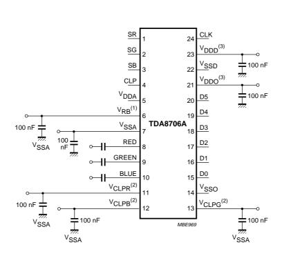
The analog and digital supplies should be separated and decoupled.
