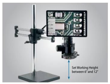
**1.** Set working height of Super-Scope® to preferred distance between 6-12". If 12"+ is required, remove lower Close-up lens.
