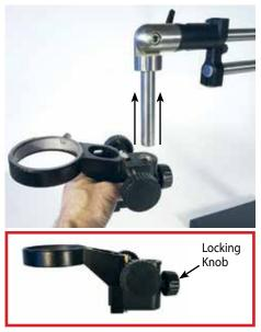
**5.** Slide microscope Focusing Mount up onto shaft. Tighten the Locking Knob lightly.
