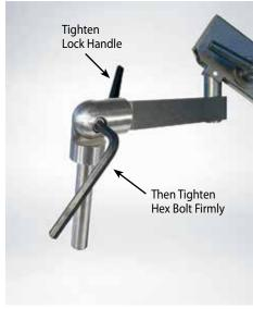
**5.** Slide Drop Arm into socket at end of Articulating Arm. Loosen hex bolt and position shaft plumb to floor. Tighten locking handle first, then **tighten hex nut very firmly**.
