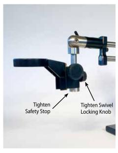
**6.** Screw Safety Stop onto end of shaft tightly. Reposition Focusing Mount down to Safety Stop and tighten. Adjust position of Focusing Mount and tighten the Swivel Locking Knob.
