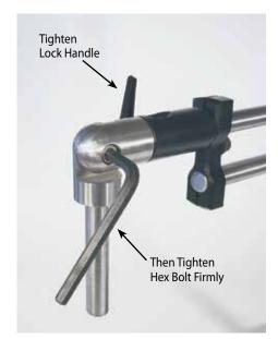
**4.** Slide Drop Arm into socket at the end of the Glide Arm. Loosen the locking bolt with the 8mm Hex Key to position shaft plumb to the floor. **Tighten very firmly.**
