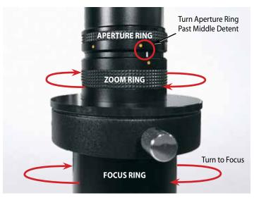
**2.** Turn the Aperture Ring to First Indicator Dot (halfway open). Then close slightly as shown (white line before indicator). Rotate the Zoom Ring to its highest zoom setting. Turn the Focus Ring until image on screen is in focus.
