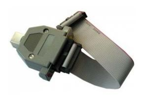
ARM debugger with JTAG and SWD interfaces, based on CoLinkEX
