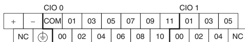
●Input Terminal Arrangement for CPU Unit with 40 I/O Points
