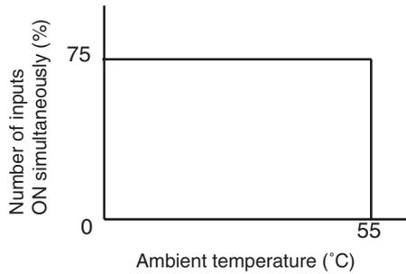
4. According to the ambient temperature, there are restrictions on power supply voltage and output load current for the CPU Units connected with the Expansion I/O Units (CP1W-8ER/16ER/20EDR1/32ER/40EDR). Use the PLC in the range of the power supply voltage and output load current as show below.
