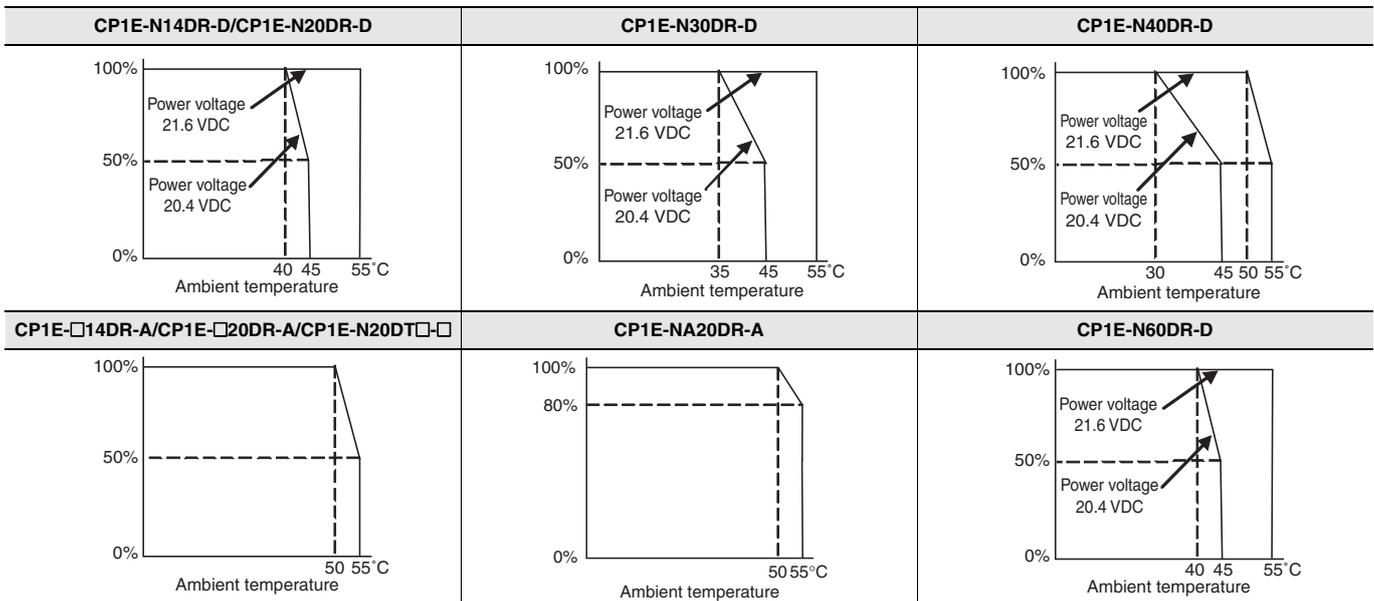
**Note:** The above restrictions apply to the relay output load current from the CPU Unit even if Expansion I/O Units are not connected.
