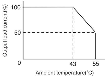
3. CP1W-32ER's maximum number of simultaneously ON output points is 24 (75%).
