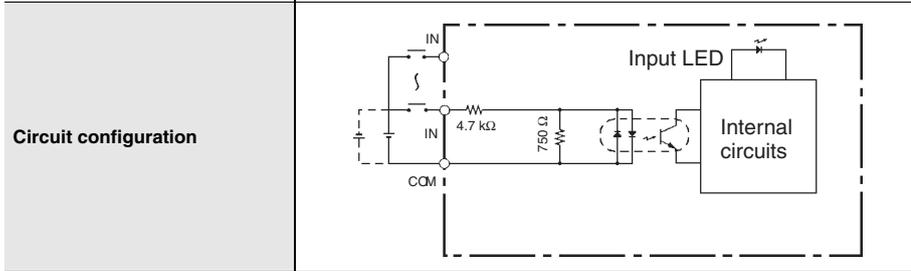
**Note:** Do not apply voltage in excess of the rated voltage to the input terminal.
