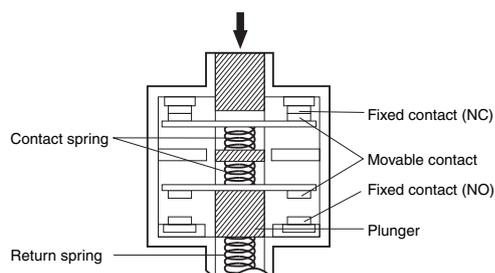
Conforms to EN60947-5-1 Direct Opening Operation ⊖
