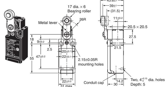
**Note:** Unless otherwise specified, a tolerance of  $\pm 0.4$  mm applies to all dimensions.
