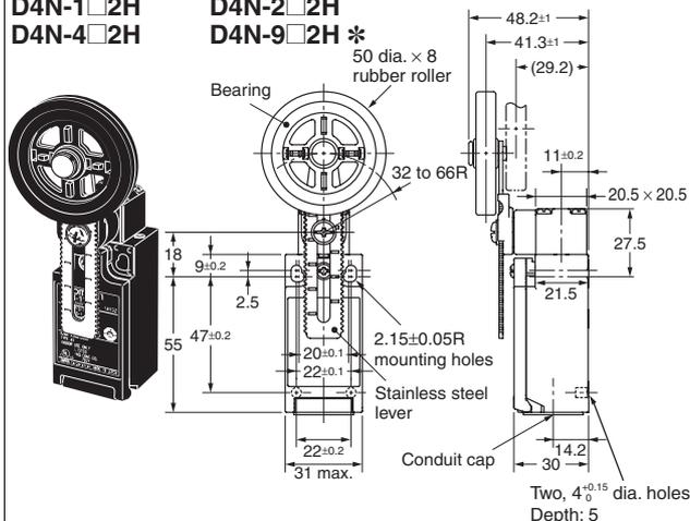
**Note:** Unless otherwise specified, a tolerance of ±0.4 mm applies to all dimensions.
