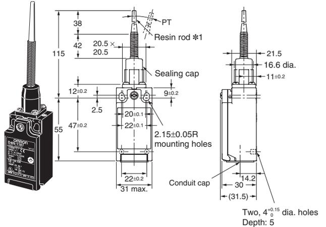
Note: Unless otherwise specified, a tolerance of ±0.4 mm applies to all dimensions.
