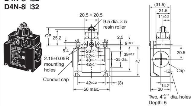
Note: Unless otherwise specified, a tolerance of ±0.4 mm applies to all dimensions.
