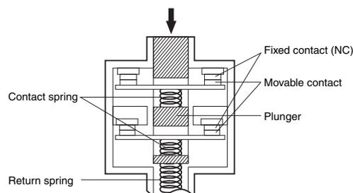
Conforms to EN60947-5-1 Direct Opening Operation ⊖
