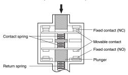
Conforms to EN60947-5-1 Direct Opening Operation ⊖
