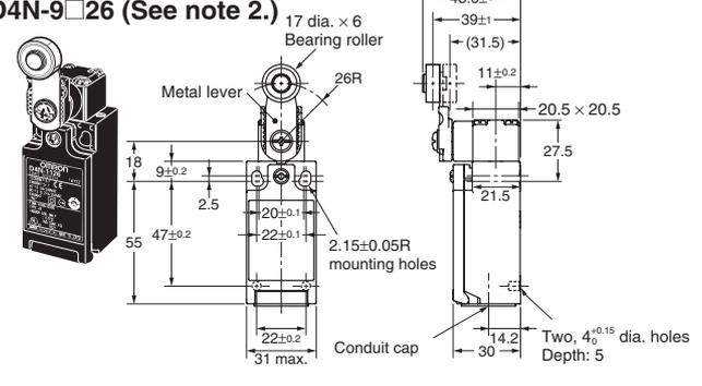
Note: 1. Unless otherwise specified, a tolerance of ±0.4 mm applies to all dimensions.
