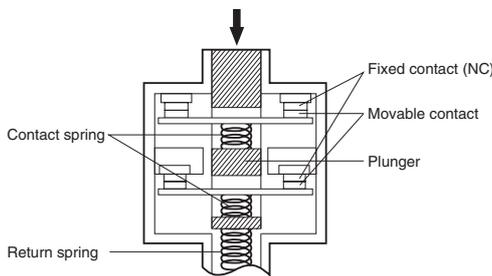
Conforms to EN60947-5-1 Direct Opening Operation ⊖
