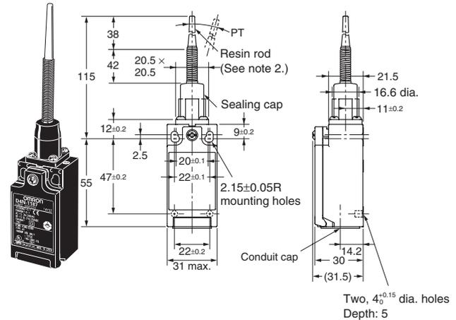
Note: 1. Unless otherwise specified, a tolerance of ±0.4 mm applies to all dimensions.
