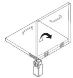
**Note:** Install the arm lever so that it will not rotate more than 180°.
