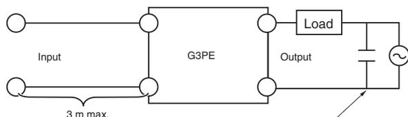
Recommended Capacitor (Film Capacitor)
