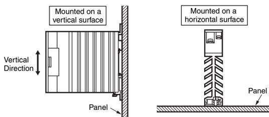
**Note:** Make sure that the load current is 50% of the rated load current when the G3PE is mounted horizontally. For details on close mounting, refer to the related information under performance characteristics. Mount the G3PE in a direction so that the markings read naturally.
